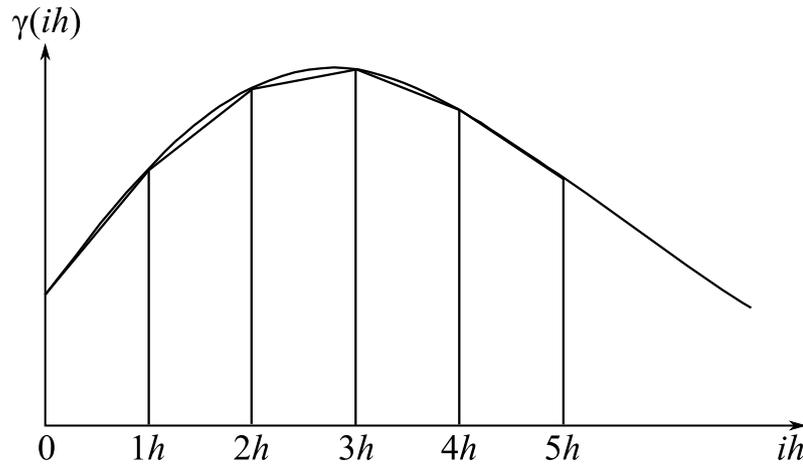
Figure 4.4: When using the trapeze rule, the area beneath the function is determined by adding up the area of the trapezes with step width  $h$  as well as side lengths  $\gamma(ih)$  and  $\gamma([i-1]h)$ .
